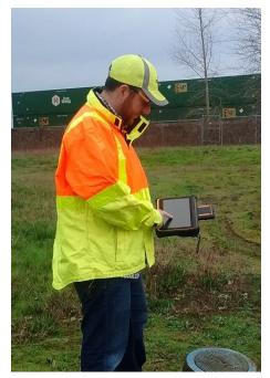
Survey grade positioning tablets are being used by ODOT construction personnel and other non-surveyors to determine "line and grade" on modern stakeless Automated Machine Guidance (AMG) jobsites. The tablets allow construction inspectors to have the same data and information that the advanced automated equipment is using to build a project.
